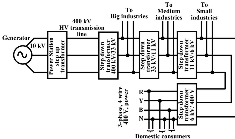
Figure 2.6: Typical voltage levels in a power system.
