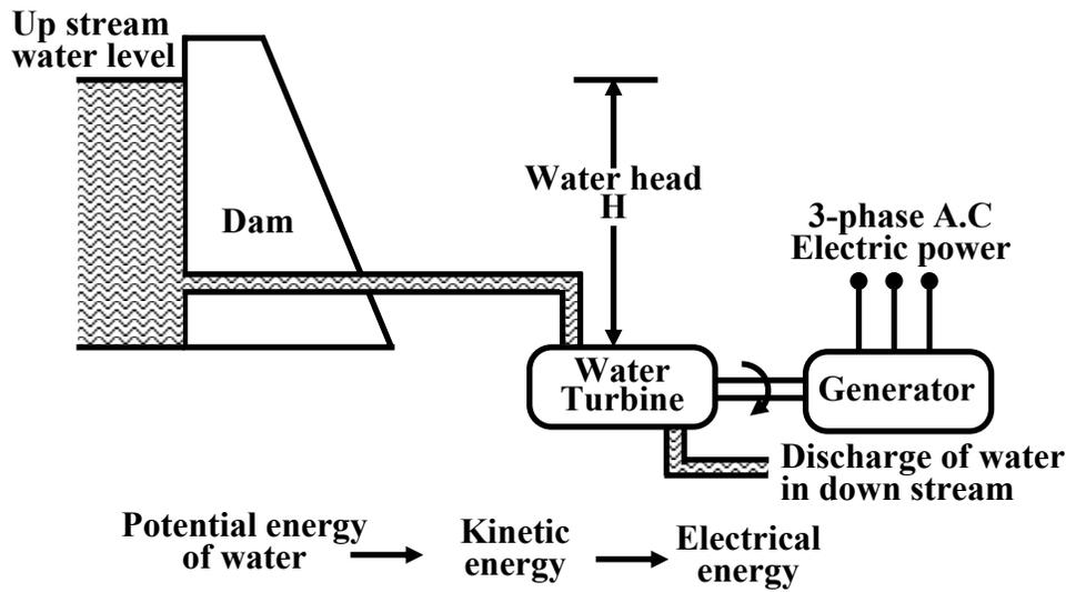
Figure 2.3: Basic components of a hydel generating unit.
