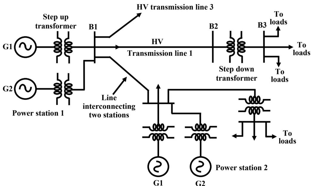
**Figure 2.10: Single line representation of power system.**
