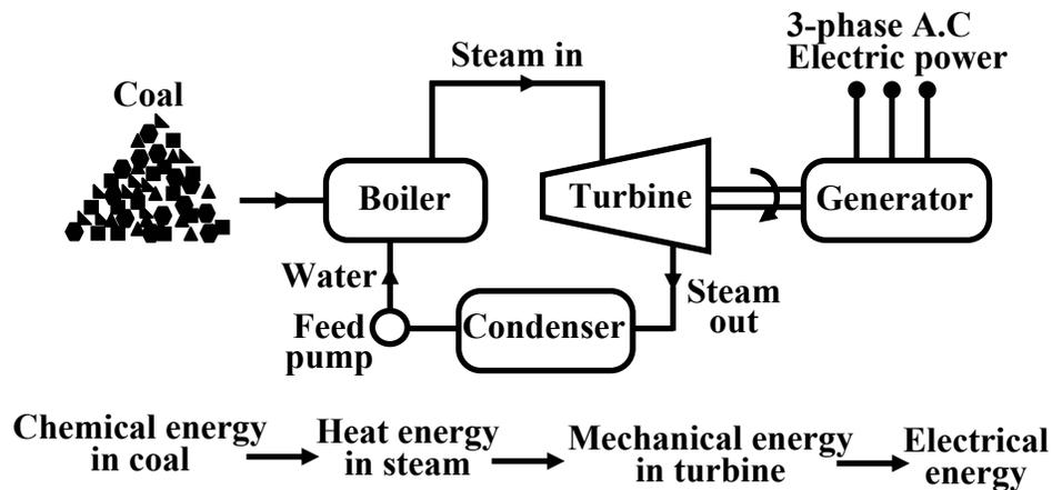
Figure 2.2: Basic components of a thermal generating unit.
