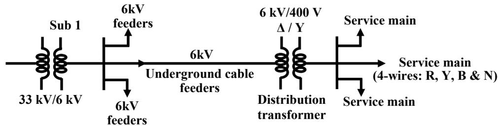
**Figure 2.11: Typical Power distribution scheme.**
